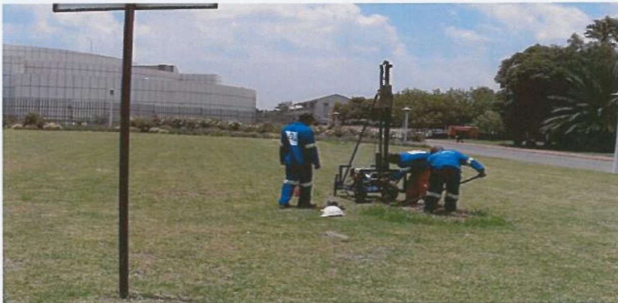
Figure 3: A Typical DPSH Test Rig from the GEOMECHANICS GROUP
